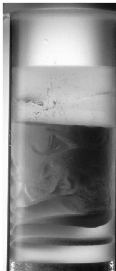
Fig. 3. Photograph illustrating the bed destruction following a change in solvent from methanol to carbon tetrachloride.
